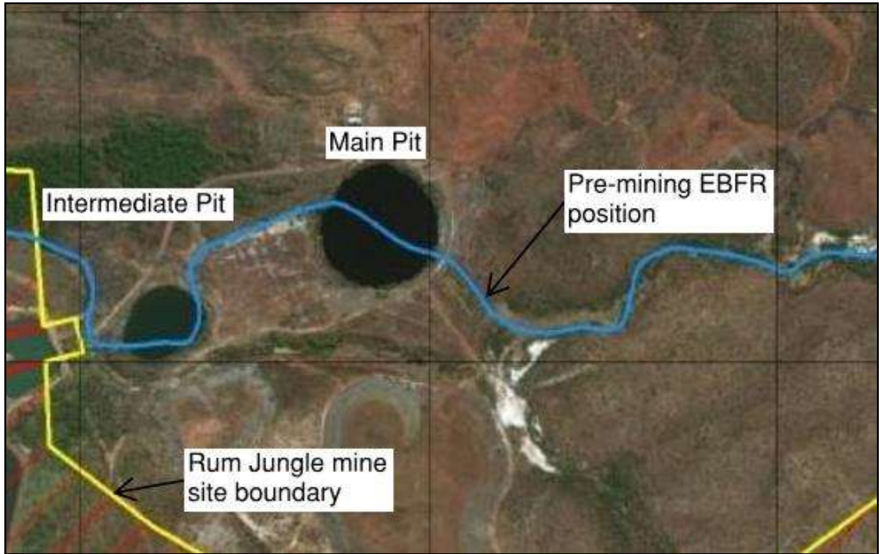
Figure 29 Pre-Mining EBFR Alignment
