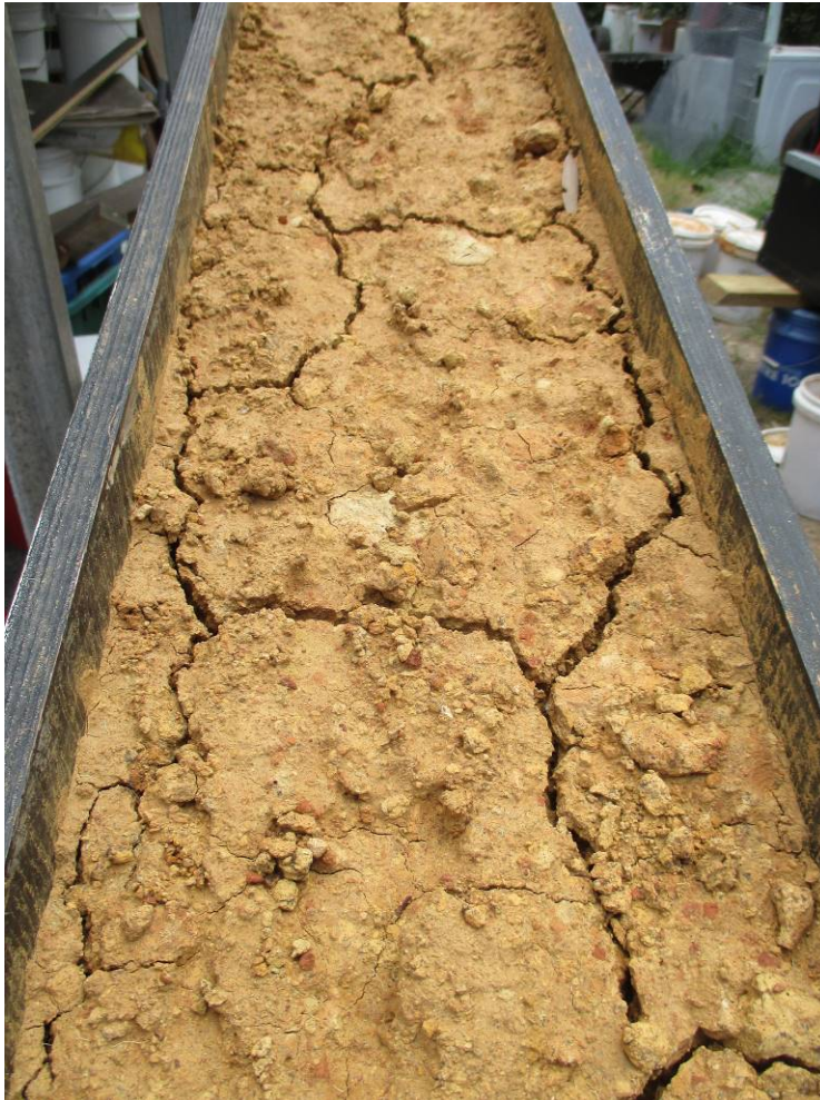
Figure 19. NPT01 4.9m-5.3m (Tan) material one week after the completion of the flume runs. Extensive cracking is evident.
