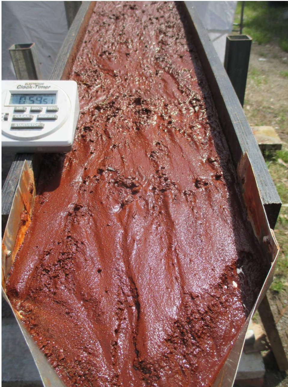
Figure 8. NPT01 0.5m-1.1m (Red) material with eroded material deposited at the outlet of the flume at the end of the 5% run.
