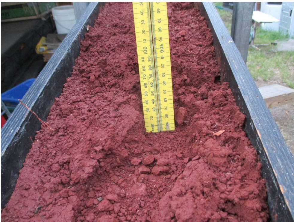
Figure 10. Eroded surface at the end of the 15% run for NPT01 0.5m-1.1m (Red) material.
