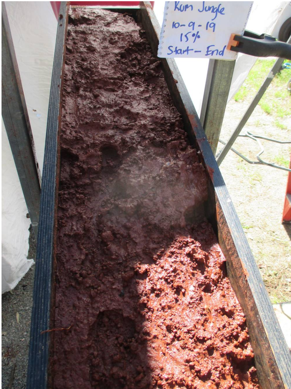
Figure 9. Eroded surface at the end of the 15% run for NPT01 0.5m-1.1m (Red) material.
