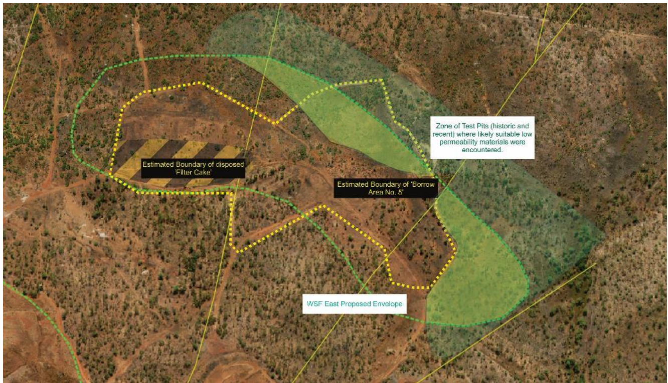
Figure 20 Old Borrow Area No. 5 Inferred Boundary and Zones of Suitable Low Permeability Materials
