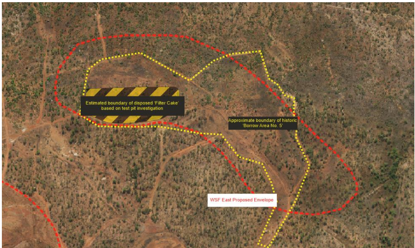
Figure 10 East WSF Envelope with Estimated Borrow Area and Filter Cake Boundaries
