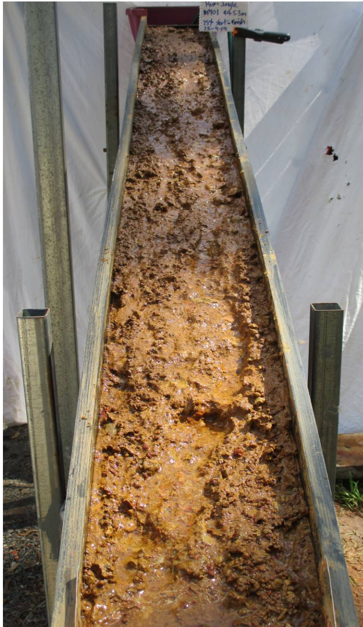
Figure 17. NPT01 4.9m-5.3m (Tan) 25% slope at the end run. Note the rill running the length of the flume.
