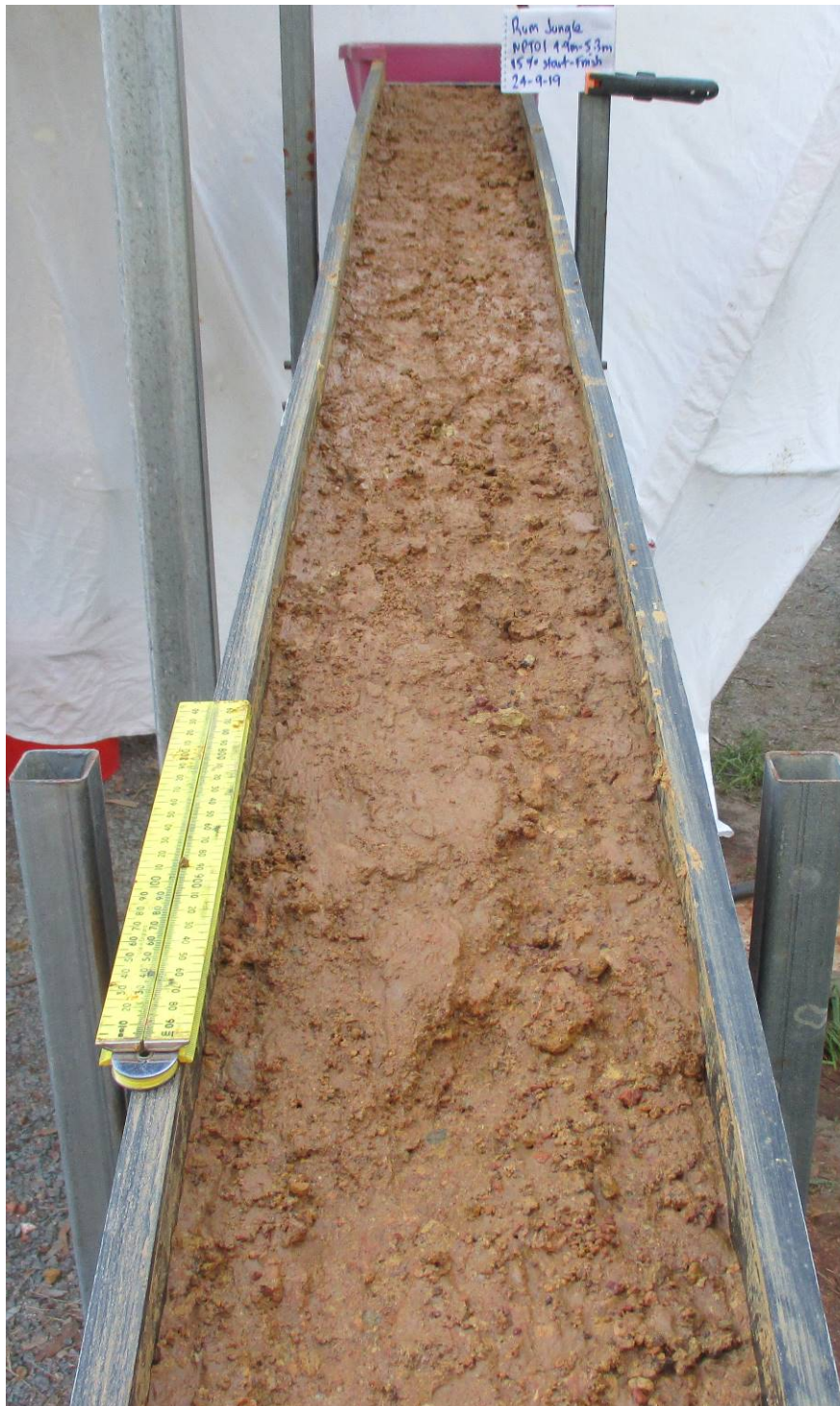
Figure 15. NPT01 4.9m-5.3m (Tan) 15% slope at the end run. Note the rill running the length of the flume.
