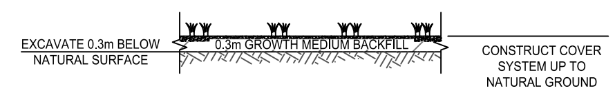
TYPICAL COVER SYSTEM OVER MT FITCH & MT BURTON WRD EXCAVATED FOOTPRINTS SCALE 1 : 100
