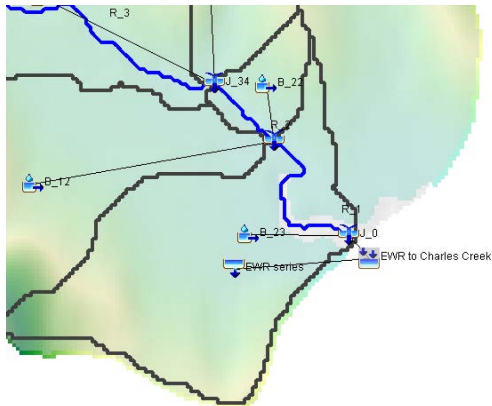
Above: Extract of Q29S HEC-HMS model (Drawing CC-01) showing the mine infrastructure catchment with environmental water release (EWR) to Charles Creek. The EWR is covers water released from the mine infrastructure to Charles Creek between 1 July 2020 to 1 July 2033 (life-of-mine). The mine site infrastructure will vary in size so the simulation comprises input from the EWRs and rainfall runoff from the area of the infrastructure catchment where no infrastructure are located.
