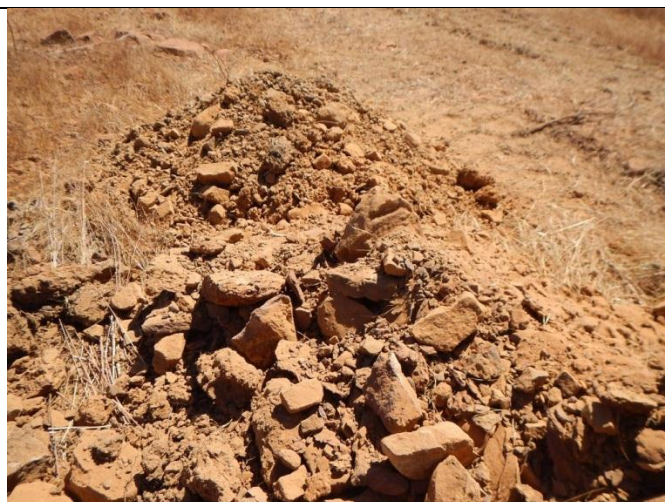
Significant coarse fragments and rock in excavations
