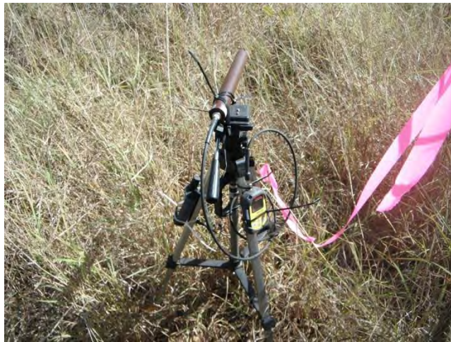
Figure 2-1 Survey meter and Garmin GPS mounted on tripod
