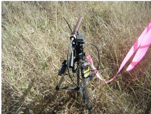
Plate 2-1 Survey meter and Garmin GPS mounted on tripod
