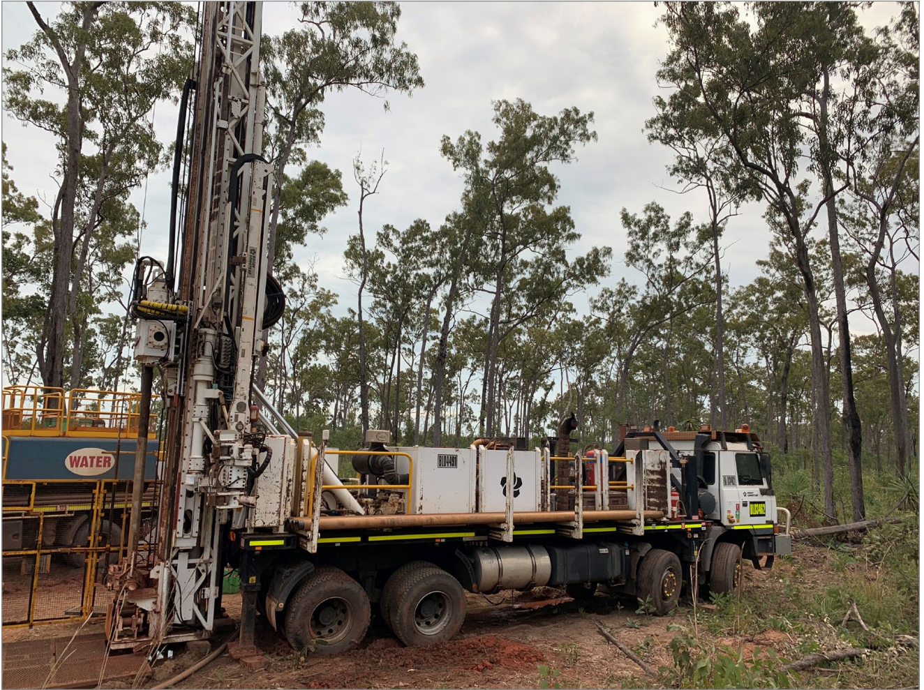
Photo 2-6 Example of a Diamond Drill Rig
