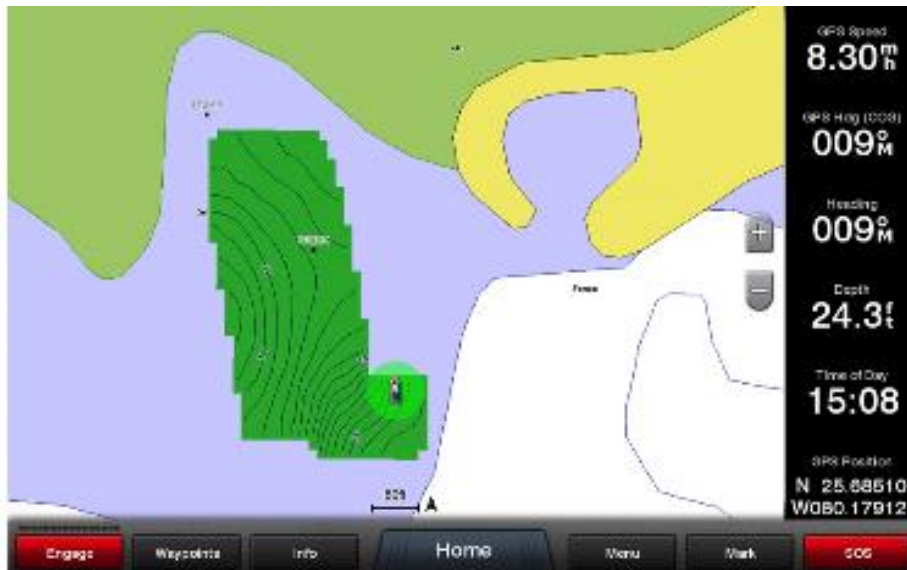
Figure 2-7: An Example of a Contour Map Created by a Readily Available GPS Sonar Device.
