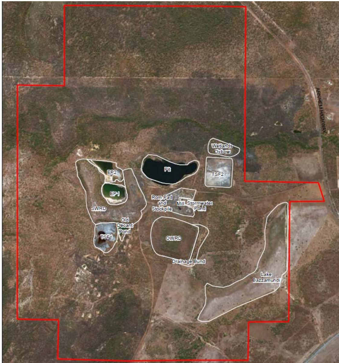
Figure 1 Layout of existing infrastructure. SWRD = Sulfide WRD; OWRD = Oxide WRD. Source: Supplement Appendix A
