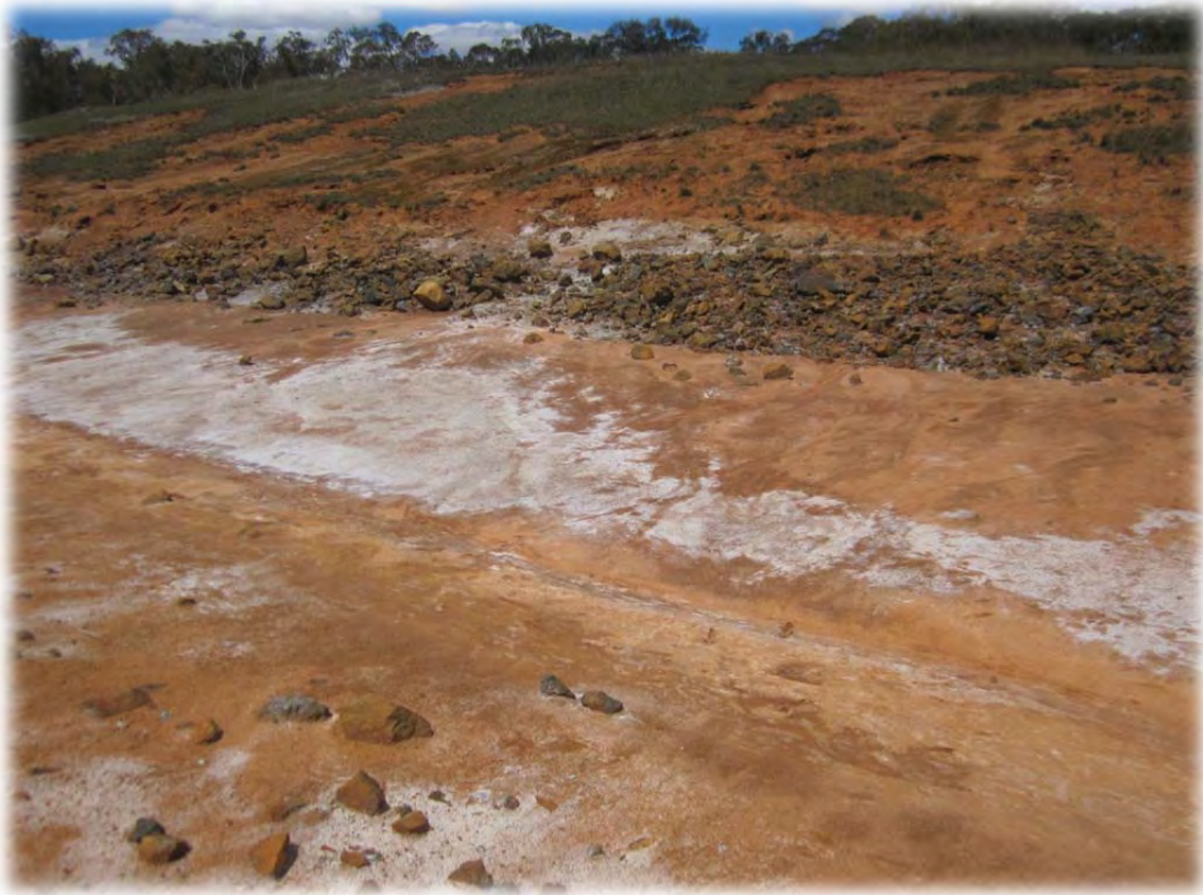
Figure 50: Secondary salt formation on a leaching waste rock dump 2
