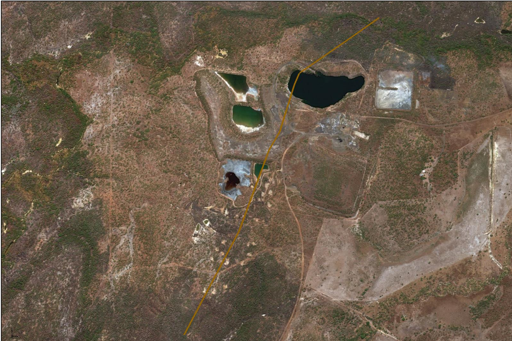
Figure 6-2 Williams Fault horizontal flow barrier (brown line)
