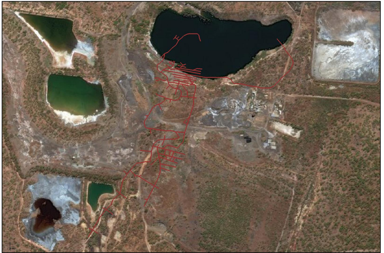
Figure 6-10 Underground workings GHB
