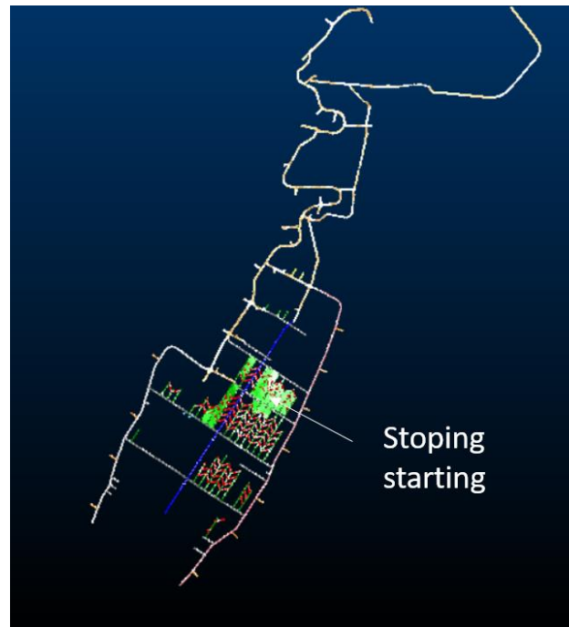
Figure 10: End of Twelve Months Extracting Ore and Accessing the Southern Side of the Orebody
