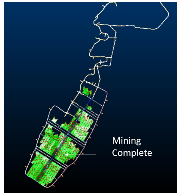
Figure 14: End of 36 Months Mining of the Lower and Upper Orebody Sections of the Orebody Completed.
