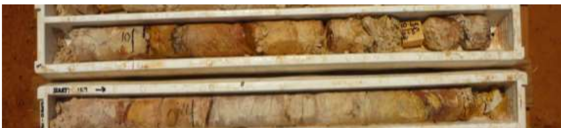
Figure 7. Typical Oxidised Siltstone samples from OPDD100004 (10-12 depth).
