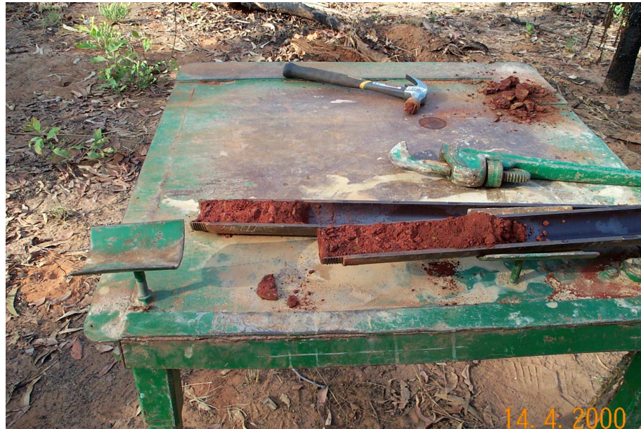
Plate 16: Core collected and sampled from the proposed plant site (Area B).
