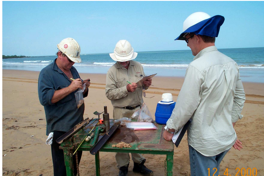
Plate 5: Logging and collection of geotechnical samples - beach area.
