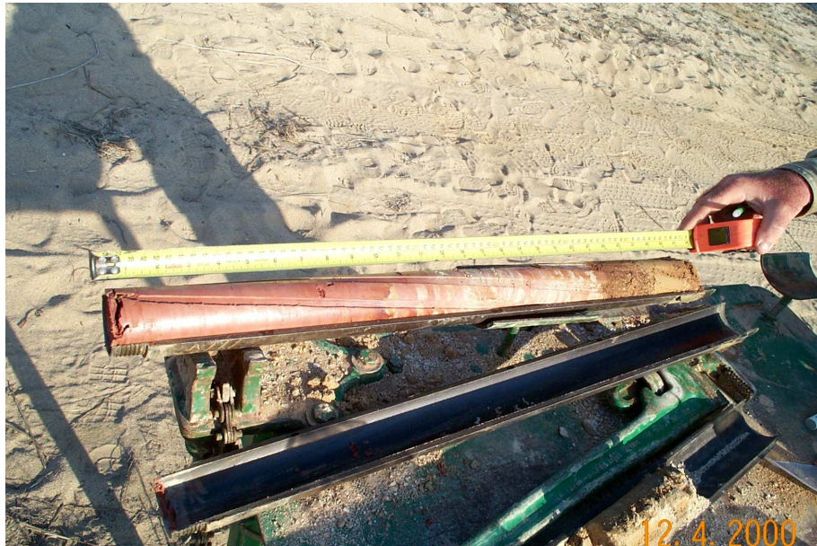
Plate 8: Core collection from OSA17 (Geotechnical Bore ID:P/BH6); 5.0 - 6.0 mbgs.
