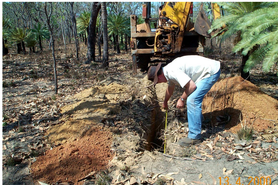
Plate 13: Measurement of test pit depth at OSB20 (Geotechnical Bore ID: P/TP12).
