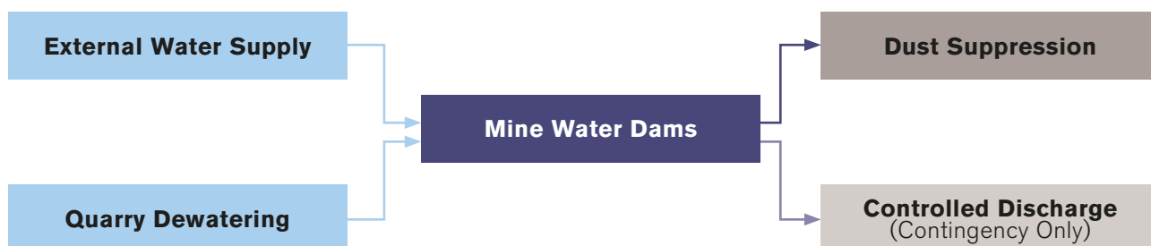
DIAGRAM 2 CONCEPTUAL WATER MANAGEMENT SYSTEM
