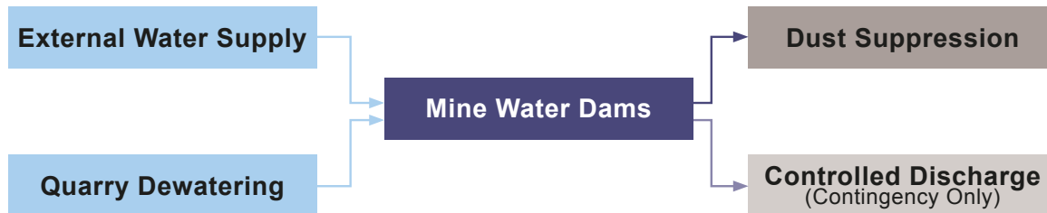
Diagram 19-1 Conceptual Water Management System for the Project
