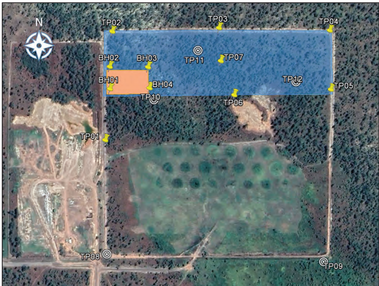
Figure 3-2 Overview of Test pits and borehole locations at Jabiru – Power Station
